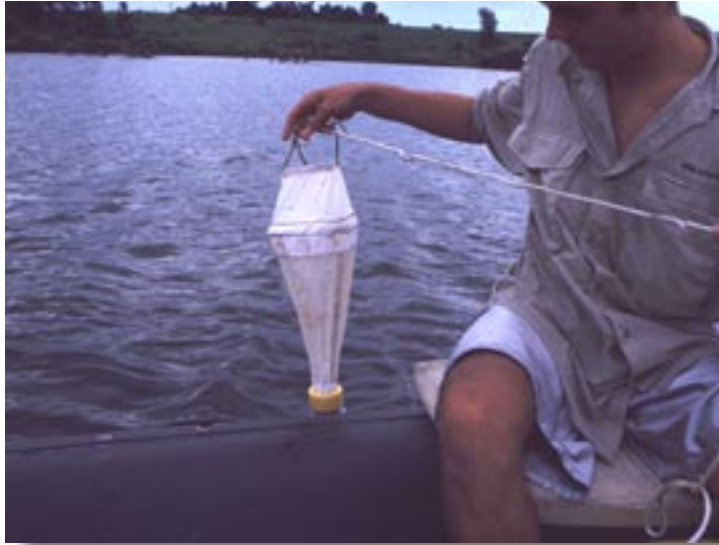
Cyanobacteria samples are often taken with a tow net at the same time as phytoplankton and zooplankton samples.
