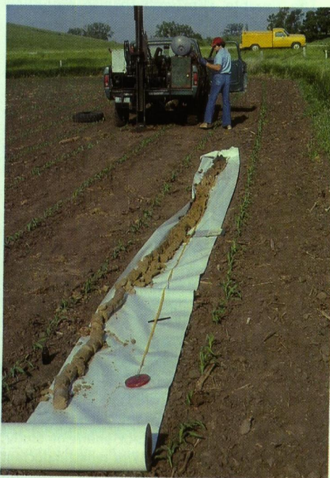
Core of Little Sioux alluvium ready for study. Photo by Bernard Hoyer.
