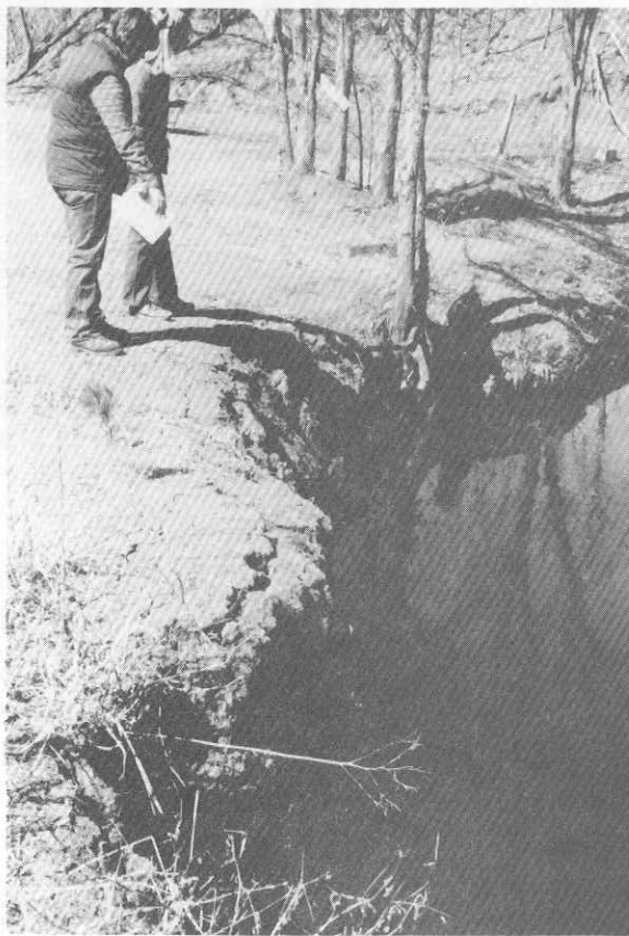
Photo No. 8 Undermined tree, steep bank, ground cracks on edge of water-filled crater, NW, NE, Sec. 9, T76N, R13W. View is roughly northwest.
