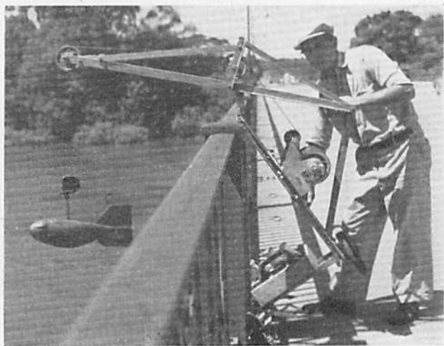
B. CRANE-MOUNTED SEDIMENT SAMPLER USED FOR CROSS-SECTIONS.
