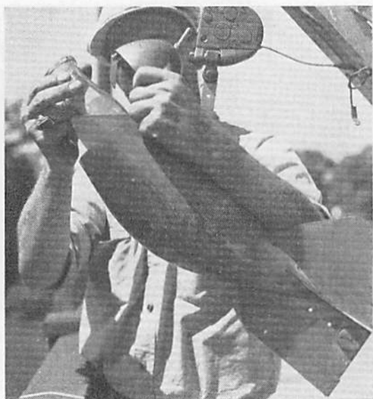
A. REMOVING SEDIMENT SAMPLE FROM U. S. D-43 SAMPLER.
