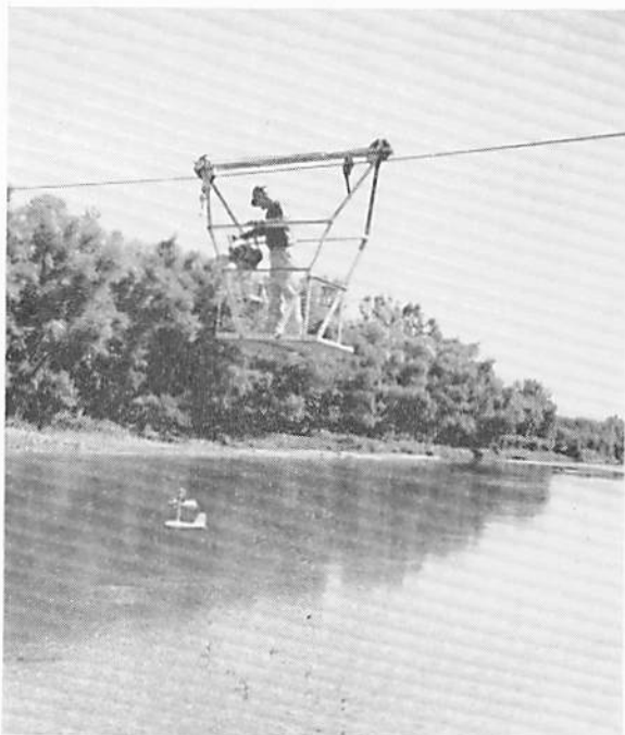
A. CABLEWAY AND MEASURING EQUIPMENT USED ON WAPSIPINICON RIVER NEAR DE WITT, IOWA
