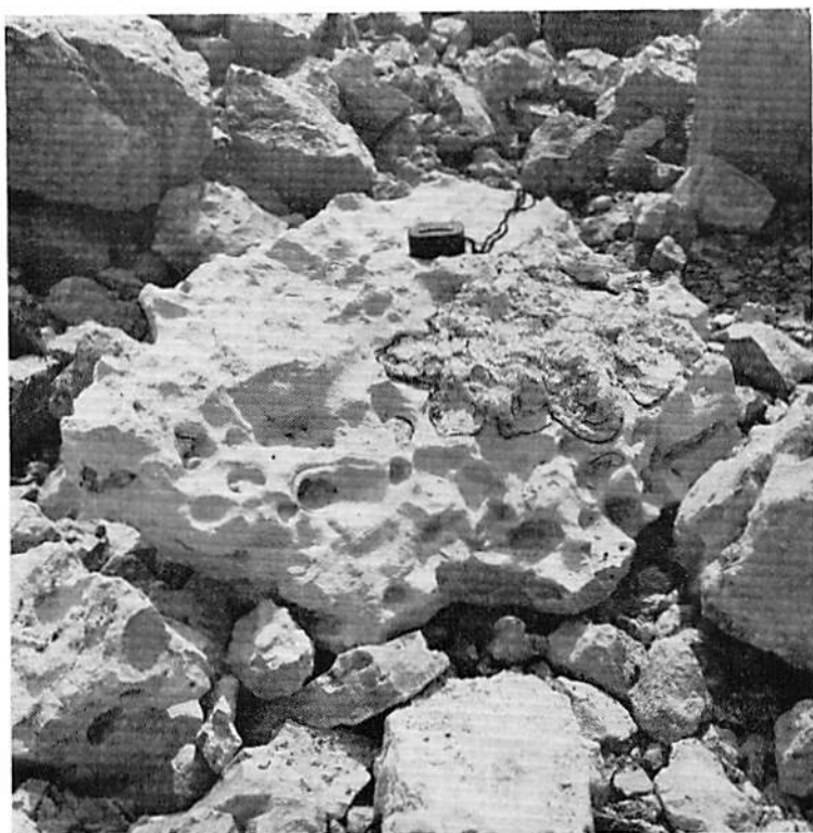
Figure 10. Typical solution-pitted Le Claire boulders displaying knobs and pits, some clay remains, Sneekloth quarry, Cedar County.
