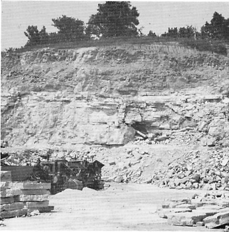
Figure 3. Quarrying operation at the Weber Company Stone Quarry, Stone City, Jones County, Iowa. This quarry is operated in the Anamosa facies of the Gower Dolomite. The evenly bedded dimension stone in the foreground is typical of the unit.
