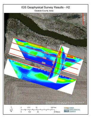
**Figure 11b.** Geophysical cross sectional locations and electrical resistivity profiles near Well H-2.
