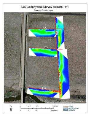
**Figure 11c.** Geophysical cross sectional locations and electrical resistivity profiles near Well H-1.
