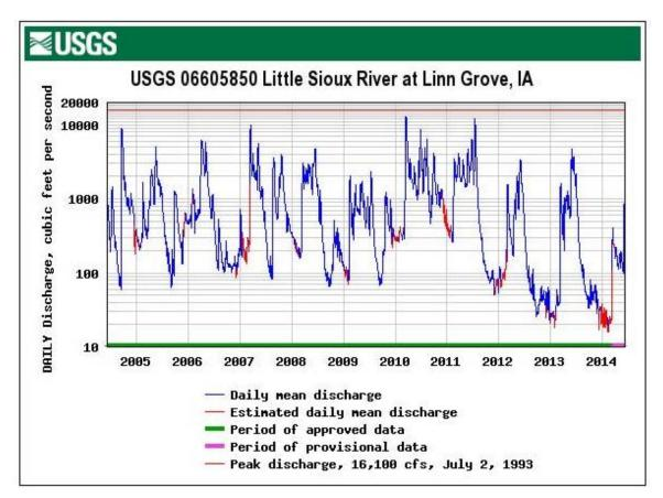
**Figure 4.** Daily average streamflow at USGS Streamgage 06605850 on the Little Sioux River at Linn Grove (2005 to 2014).
