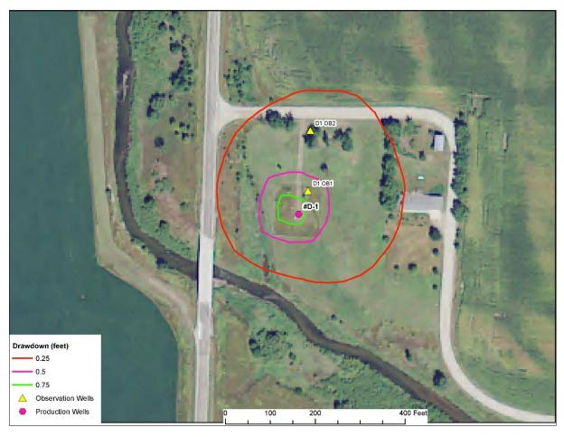
Figure 12. Simulated drawdown near well D-1 used in model calibration in Table 10.
