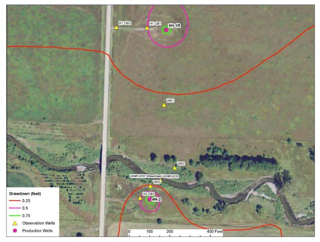
Figure 13. Simulated drawdown near H-Series wells used in model calibration in Table 10.
