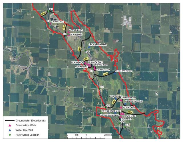
Figure 7. Observed groundwater elevation contours for Osceola County Rural Water District and surrounding area.
