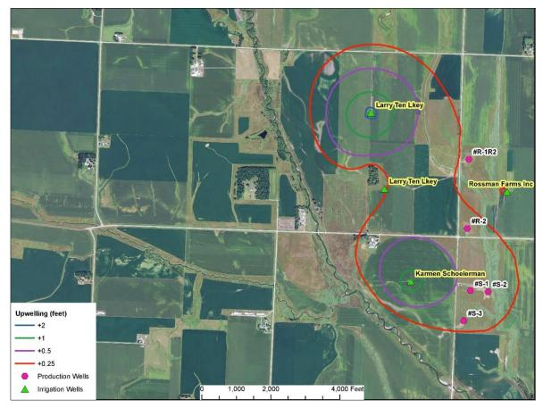
**Figure 20.** Simulated upwelling in the groundwater table if the irrigation wells are shutoff near the RS-Series wells.
