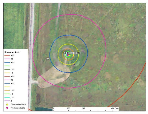
Figure 15. Simulated drawdown near RS-Series wells used in model calibration in Table 10.
