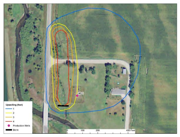
Figure 19. Proposed earthen berm location and simulated upwelling near Well D-1.
