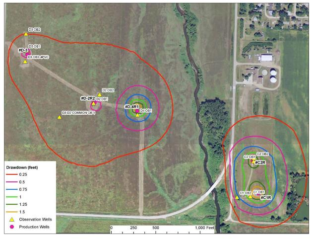
Figure 14. Simulated drawdown near the CD-Series wells used in model calibration in Table 10.
