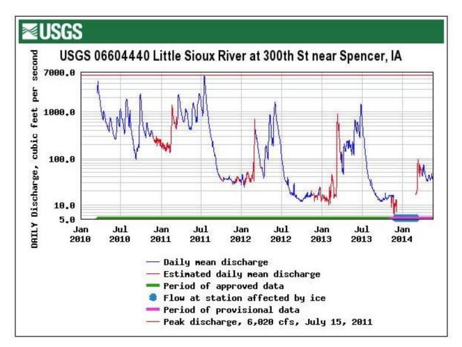
**Figure 3.** Daily average streamflow at USGS Streamgage 06604440 on the Little Sioux River near Spencer (2010 to 2014). USGS began collecting streamflow in 2010.
