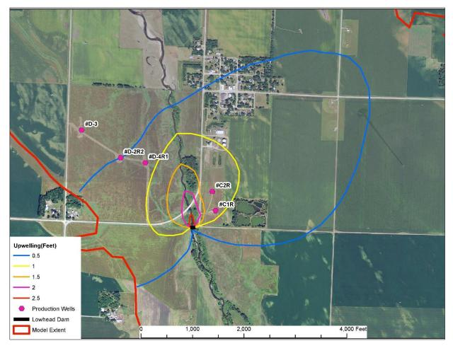
Figure 17. Proposed low head dam location and simulated upwelling (rise in water table) near the CD-Series wells.
