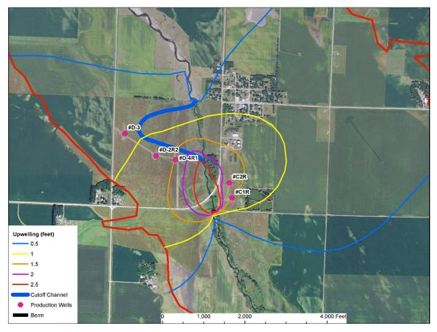
**Figure 18.** Proposed low head dam location and simulated upwelling (rise in water table) near the CD-Series wells with the addition of a proposed cutoff channel.
