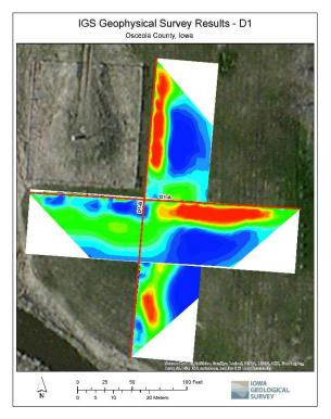
**Figure 11a.** Geophysical cross sectional locations and electrical resistivity profiles near Well D-1.
