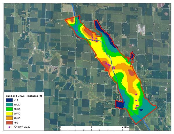
Figure 6. Sand and gravel thickness (isopach) map of the model area.
