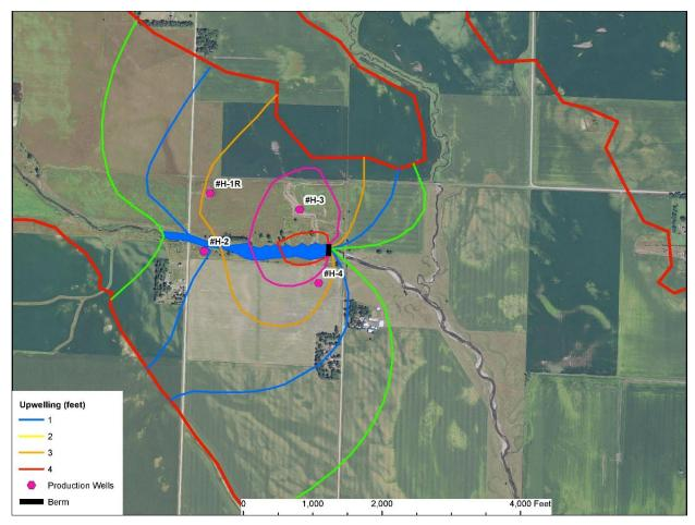
**Figure 16.** Proposed low head dam location and simulated upwelling (rise in water table) near the H-Series wells.
