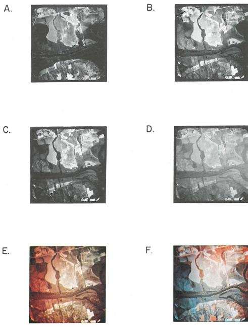
Plate 2. Five days after flood recession on a landscape cover of bare soils predominantly. All bands effectively discriminate flood boundaries on the bare soils. However, contrast is greatest with infrared band (A) and decreases with the red (B), green (C), and blue (D) bands, respectively. Color (E) and color infrared (F) adds very limited information on flood inundation in areas completely covered by bare soils.
