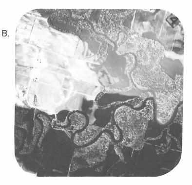
Plate 1. Comparison of red, A (595-685 nm) and infrared, B (740-900 nm) bands imaging April, 1973 flood shortly after the flood crest. The junction of the North and South Skunk Rivers represent two streams with unlike sediment load at the time these images were produced. Notice that the contrast between the soils and water is greater in the infrared band for both the high sediment load stream (North Skunk) and the low sediment load stream (South Skunk). Α.
