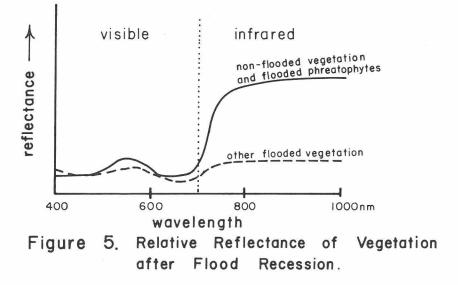
accurately mapped, even under the high soil-moisture conditions that would normally occur in the Midwest during the spring (Hoyer, et al., 1974). Bare soils located in areas having a high potential for evaporation may show a decrease in reflectance for a shorter time interval, however, sufficient data has not been gathered on this problem.
