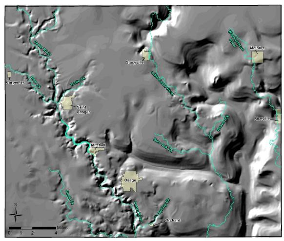
Figure 5: Raster image of the bedrock surface of Mitchell County using "hillshade" effect. Image generated from the bedrock topography lines drawn at 25-foot contour intervals.
