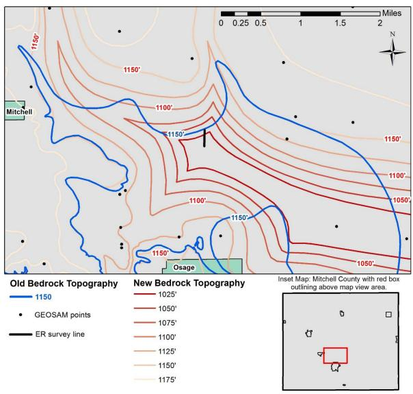
Figure 3: Comparison of a portion of the old and new bedrock topographic maps.
