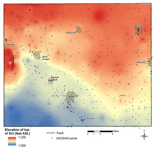
Figure 6: Raster image of the elevation of the top of the Coralville Formation. "U" and "D" indicate the upthrown and downthrown sides of the fault, respectively.
