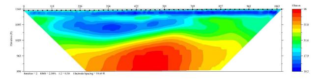
Figure 4: South (left) to north (right) cross-sectional view of the ER model from the area shown in Figure 3 (black line). Warm colors indicate competent bedrock. Depth is shown as elevation in feet above sea level on the X-axis.
