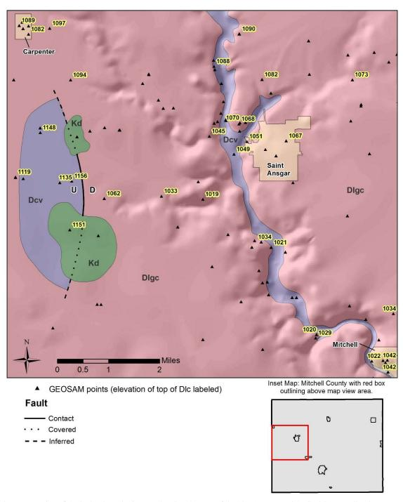
Figure 7: Portion of the bedrock geologic map showing the area of the "St. Ansgar Fault". GEOSAM well points are labeled with the elevation of the top of the Little Cedar Formation. "U" is upthrown side and "D" is downthrown side of the fault.
