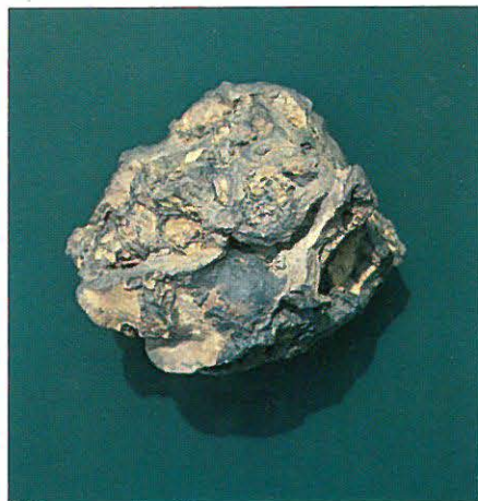
Limonite is a distinctively yellowish brown ore of iron . It takes many forms, including the cellular structure seen in this sample from the historic Iron Hill area near Waukon in Allamakee County.
