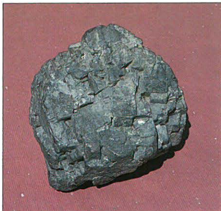
Galena has a distinct metallic-gray luster and a cube-shaped crystal form. It is very heavy and is the principal ore of lead . This mass of crystals is from Dubuque County, where lead ores were mined for over 300 years from veins in the dolomite bedrock.
