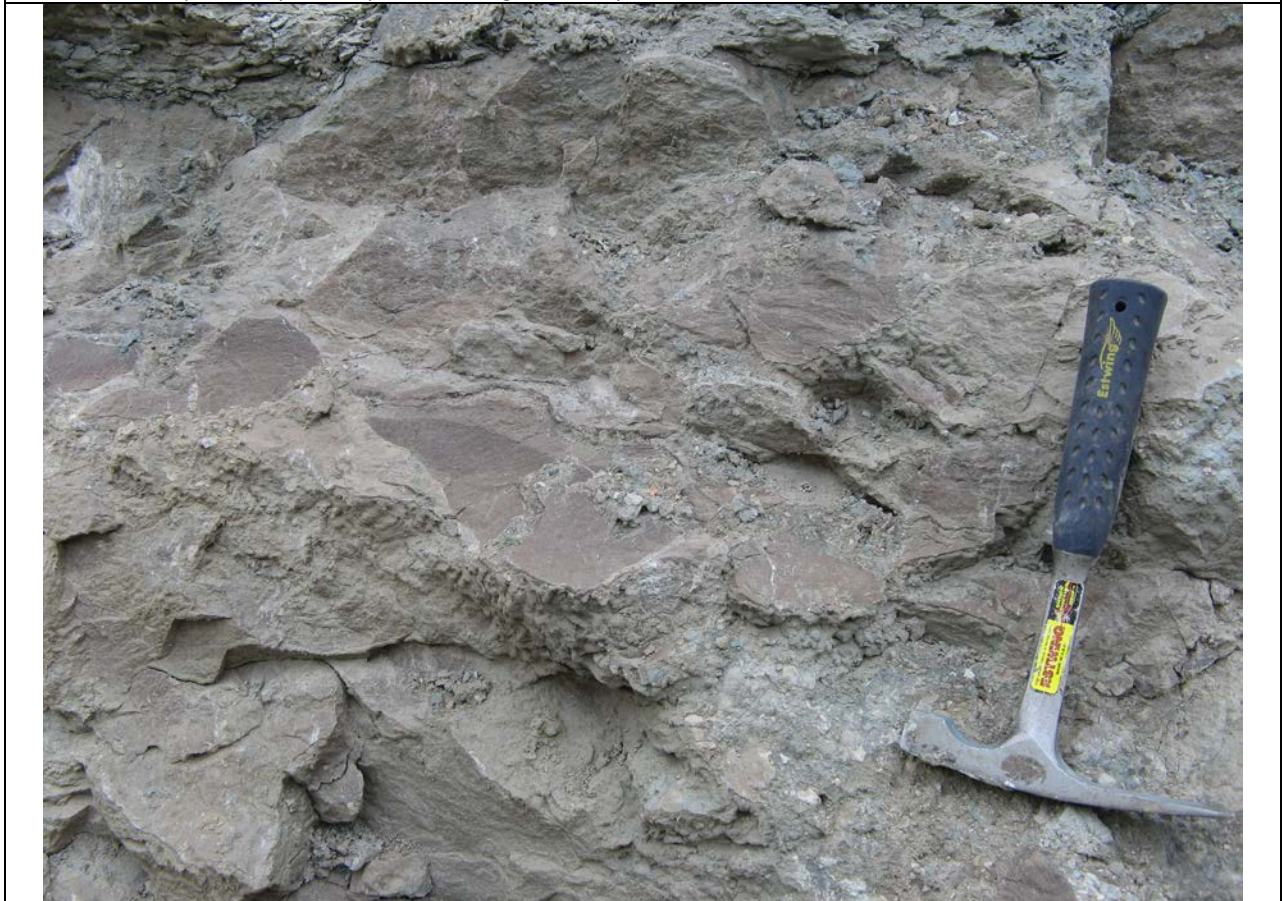
Photo 4: Brecciated dolomite of the lower "St. Louis" Formation seen in the Beach Quarry.
