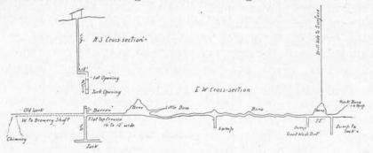
Fig. 87. Vertical cross-sections of the Bush mine, 1899.
