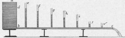
FIG. 4. Diagram illustrating relation of water pressure to distance from source.
