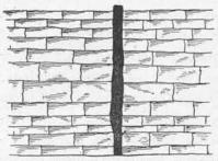
A vertical sheet, in this case carrying lead ore, is illustrated in figure 60. This sheet was sketched in the McPoland and Basler mine in West Dubuque in 1899, but similar sheets have been followed in the Avenue Top and a large number of other Vertical sheet of galena in McPol. well known mines. The simple sheet of mineral, here one-half
