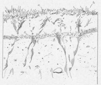
FIG. 8. Typical section through drift and losss in Lyon and Sioux counties, showing position of intervening gravel and sand layer.
