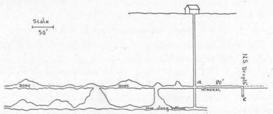
Fig. 86. Vertical east-west section of Avenue Top workings on McNulty crevice.
