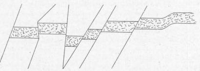
FIG. 44. Diagrams showing displacement by faulting in a single layer of clay, slightly over a foot in thickness.
