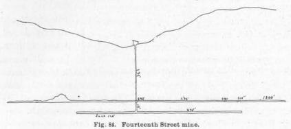
as indicated in the sketch. From the shaft a drift was run south ninety feet and yielded good dry bone all the way. East of this level, at a distance of 370 feet, a level has been run south thirty-five feet, and twenty feet beyond it a second has been carried south fifteen feet. Beyond this the crevice has been followed 1,300 feet. These various entries at this level all yielded good dry bone and show much mill dirt yet in the walls. They average about four by six in cross section,
