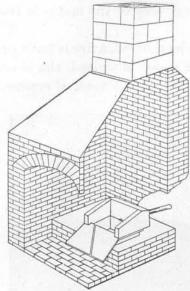
Fig. 96. Scotch hearth furnace as used at Dubuque.
