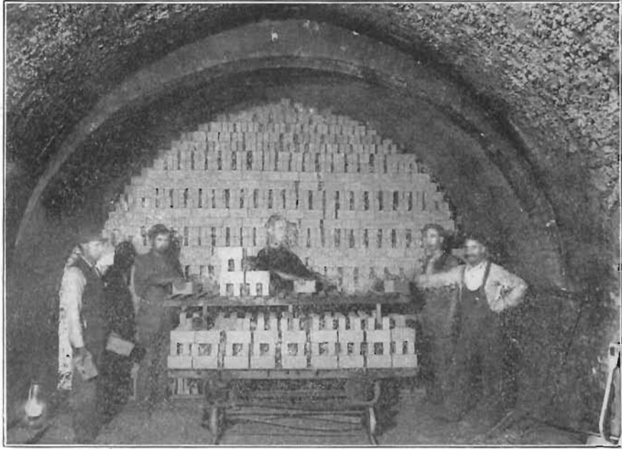
FIG. 72 Interior view of Haigh continuous kiln showing method of setting brick; Sioux City Brick and Tile Company, Sioux City Iowa.
