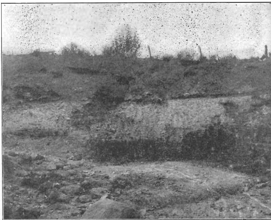
FIG. 25. G. H. Orcutt clay pit. One-half mile west of Monroe. Coal blossom and shale above a thick bed of fire clay.
