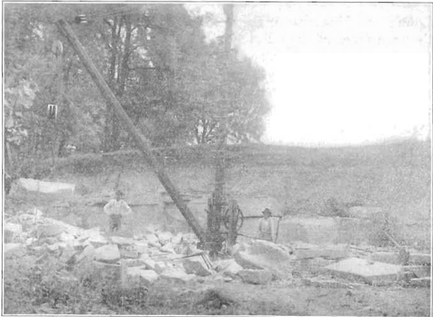
FIG. 30—Davis quarry, west of Bentonsport, Van Buren county. Heavy beds of magnesian sandstone (Warsaw Sandstone).
