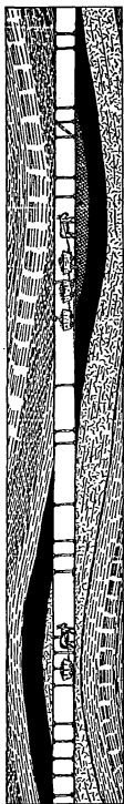
Figure 85. Section Showing Undulatory Character of the Coal Seam in Bloomfield Mine. Des Moines.
