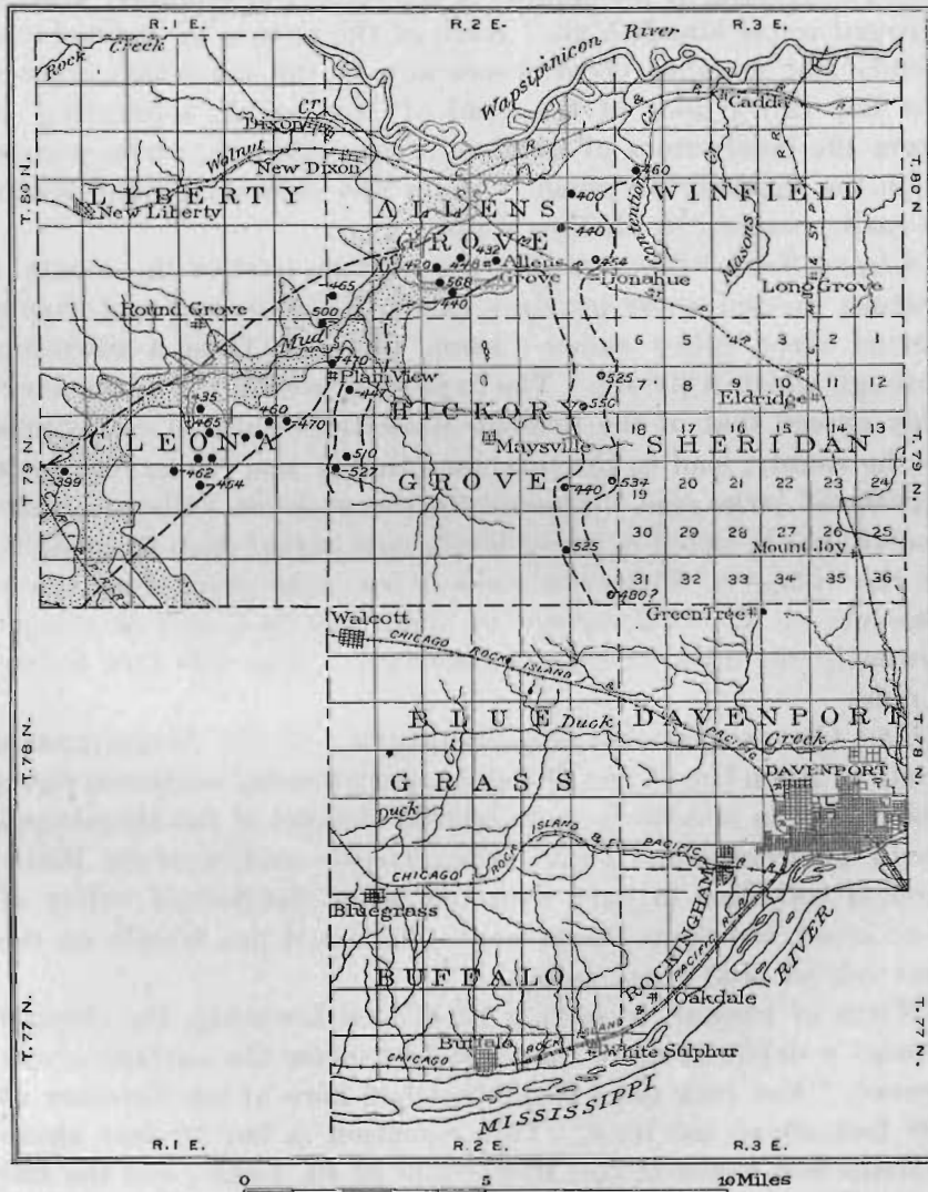
Figure 5.—Map of western Scott county, showing the ancient channel now occupied by Mud creek (shown by shading) and the buried Cleona Channel (bounded by broken lines). Figures at deep wells (●) indicate the elevation of the rock surface above sea level. Figures prefixed with minus signs are used with wells which did not reach rock and indicate that the rock surface is less than the elevation given, that of the bottom of the well.
