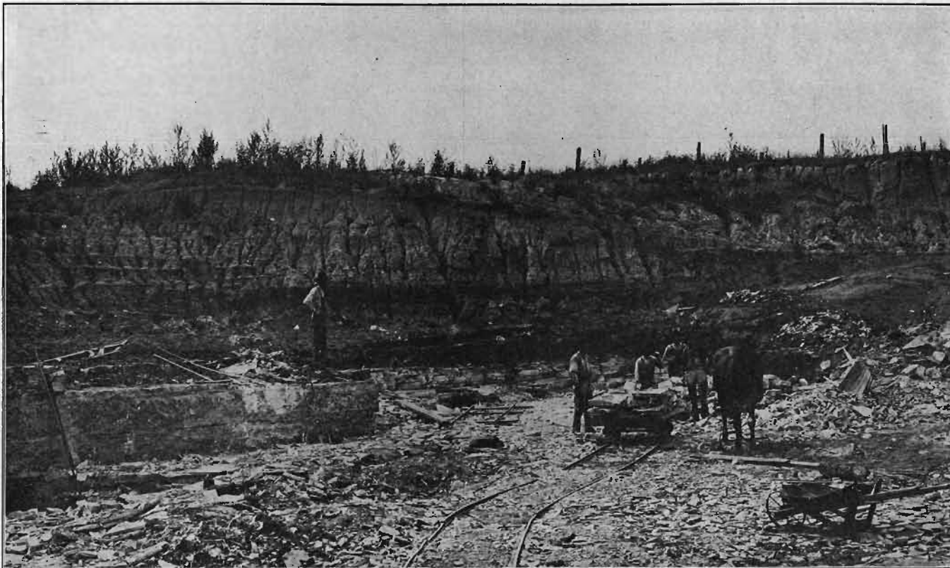
PLATE LVI—Andrew Lames quarry, Dudley, Wapello county. The section shows the hard, compact beds of the Saint Louis limestone under the usual heavy stripping of the district.
