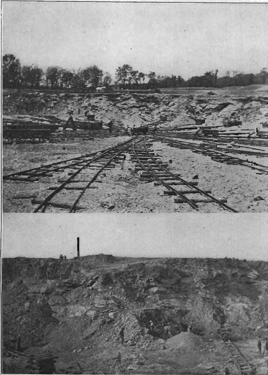
PLATE LII—Clark quarry, near Buffalo, Scott county; upper view showing track- age arrangements leading to incline, lower view showing irregular beds and large amount of shaly talus.
