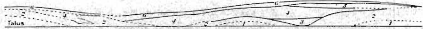
Fig. 9.—Diagram of cut on Chicago, Milwaukee & St. Paul railway east of Martelle, Iowa, showing relations of Kansan till (1 and 2); gray clay (3); Buchanan (?) gravel (4); Iowan (?) till (5); loess (6).
