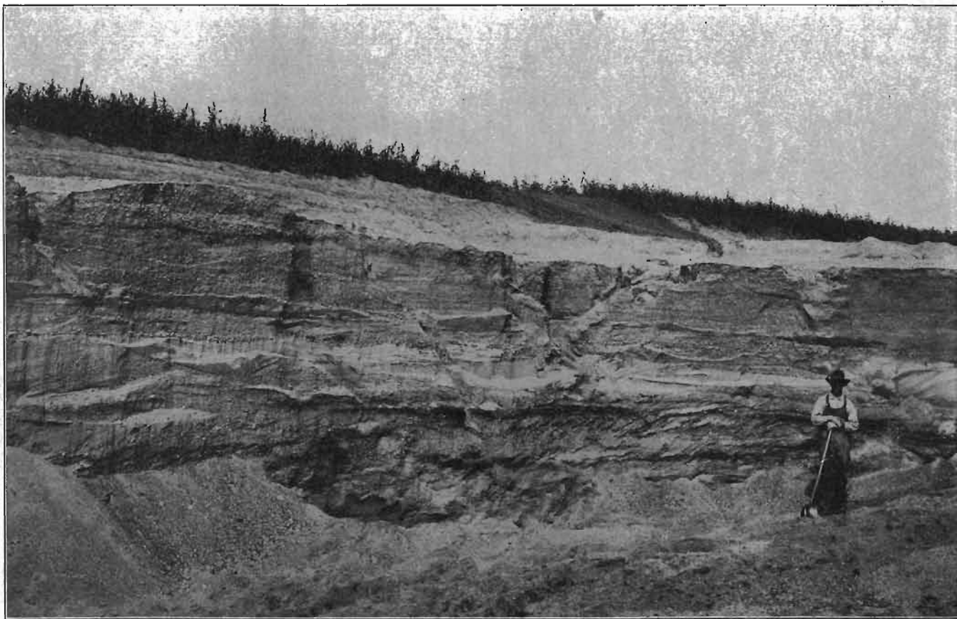
Lehatchka and Pattengill pit about half a mile north of Rock Rapids, Lyon county. The view shows cross-bedding and basin structure, variation in the coarseness of the material, and the thickness of the stripping. (Beyer, Iowa Geological Survey, volume XXIV, Plate XXXII, page 421.)
