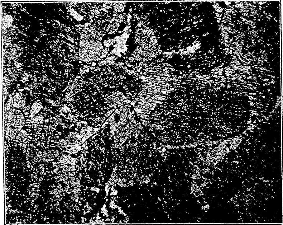
FIG. 1 Microphotograph (x 45), Burlington limestone, natural light.
