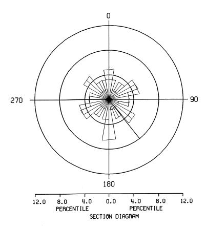
Figure 8. Rose diagram of the orientations of vertical joints that form a polygonal network in the Aurora Till Member (site 3 on Fig. 7; 31 joints from 16 contiguous polygons).
