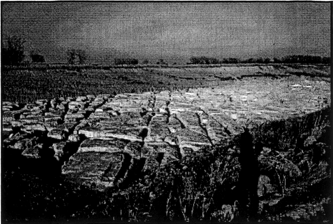
Figure 7. Photograph of the exposed gypsum in the North Welles Quarry prior to blasting and removal in 1984. The solutionally enlarged fracture system is evident.
