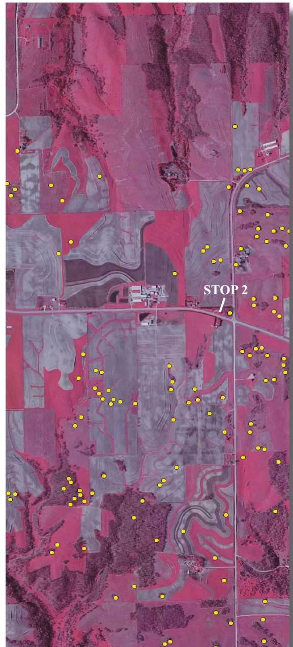
Figure 2-1. Color infrared photo of the Rossville area showing sinkholes (yellow circles).
