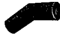
VERSA-TILE This is a slant end tile, cut at an angle of 22 1/2 degrees, designed to be used in pipes for turning corners of any angle. The slant ends are beveled together in the slope pipe elbow fashion to give any angle from 0 degrees to 45 degrees. They can be used singly, turning in starting laterals off junctions, turning in corners, or any use where change of direction is desired. A Rockford invention. Available in all sizes from 4" to 12".
