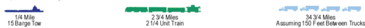
Figure 8. Comparison of carrying capacity and size of river barges, trains, and trucks.
