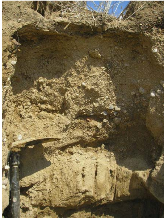
Figure 3 Matrix-supported pebble gravel overlying channel fills of laminated deformed silts and fine sand. Shovel placed at contact.
