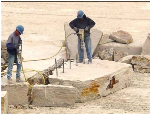
Figure 8. The stone is then split into manageable size blocks by hand.
