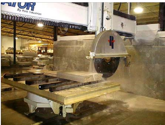
Figure 10. Other blocks are sawed to specific shape using one of a variety of water-cooled saws.
