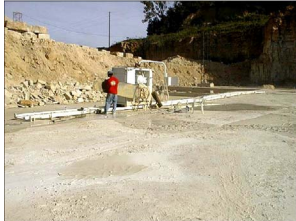
Figure 7. The rock is sawed into strip with a ledge saw.
