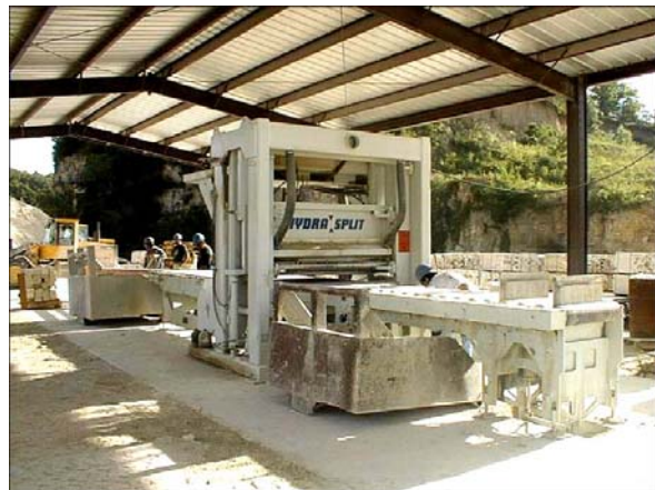
Figure 9. Some blocks are split to specific size with hydraulic cutter.
