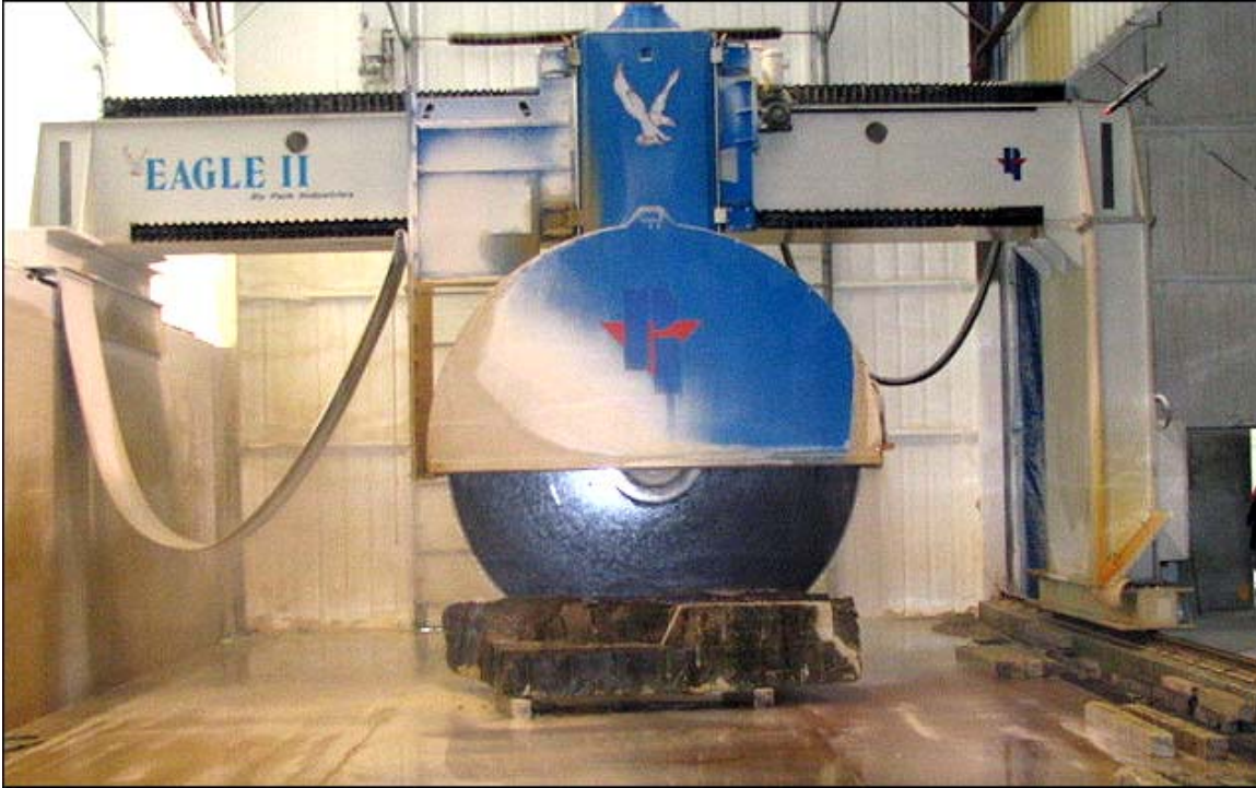
Figure 3. Photograph of the largest rock saw at the Weber Stone Company's rock finishing building at Stone City. Photo by Thomas Marshall.
