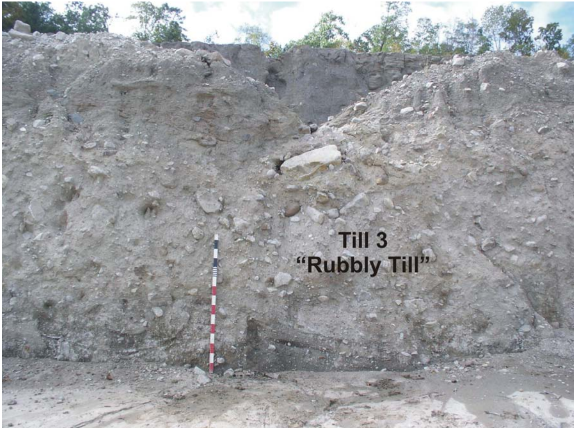
Figure 8. Lowest Pre-Illinoian bench at Moscow Quarry. Approximately ten feet of a Till 3, a rubbly clay loam diamicton rests unconformably on Devonian age bedrock. Many of the clasts are locally derived. Photo by Kathy Woida.
