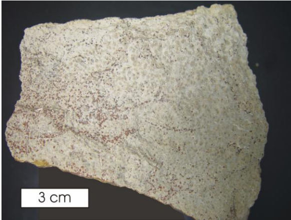
Figure 5. Photograph of hand sample of calcite concretion with contained sphaerosiderites visible as dark spots from their contained pseudomorphic iron oxides. From Melcher-Dallas locality in southwestern Marion County, Iowa. This sample comes from a siliciclastic mudstone paleosol (underclay) in the Laddsdale coal interval from the lower Floris Formation (Desmoinesian) of the Cherokee Group.
