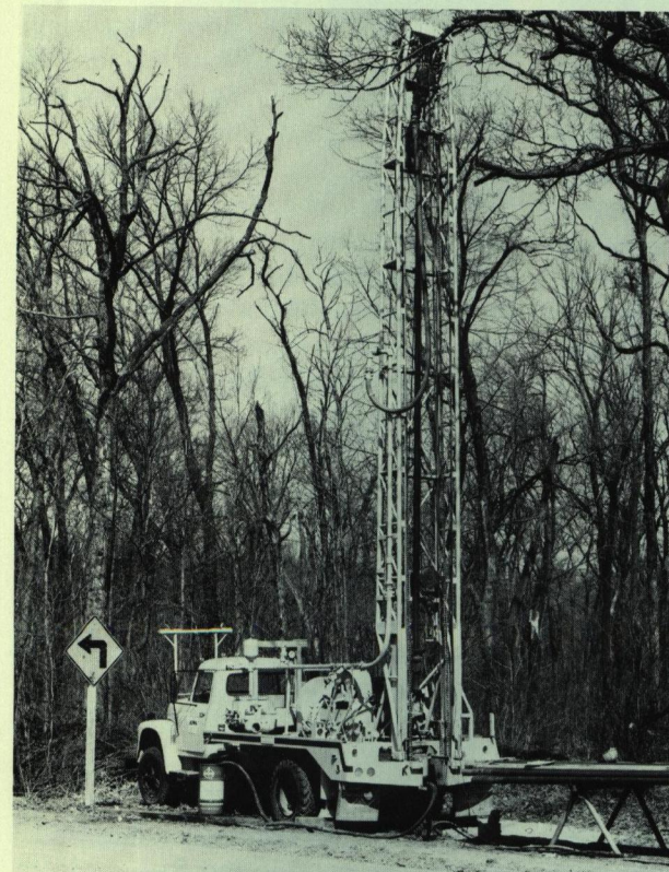
pumping Test drilling for the Carbonate Hydrology Project with the Survey's Failing #1250 rotary rig.
