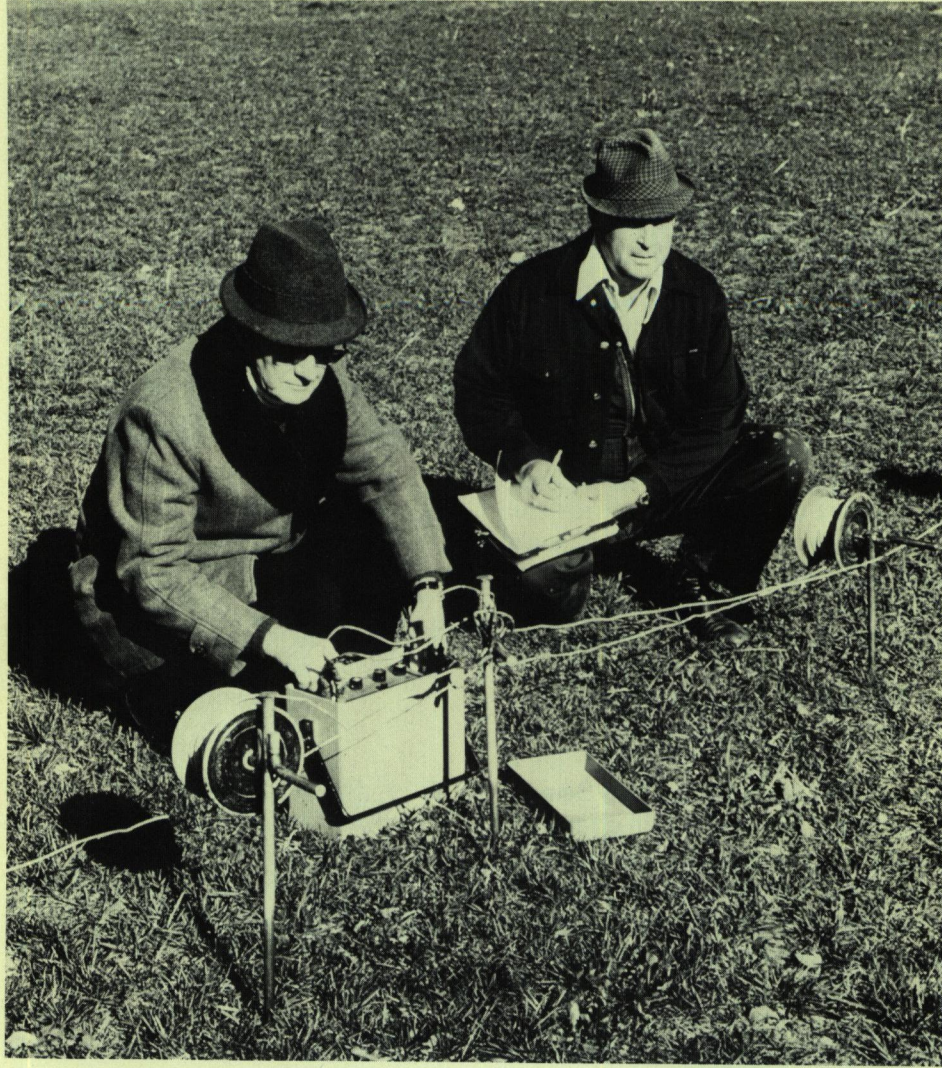
Resistivity used for subsurface research
