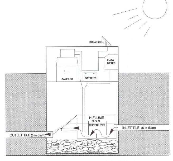
Figure 8. Diagram of monitoring sumps at L22T and BTLD.
