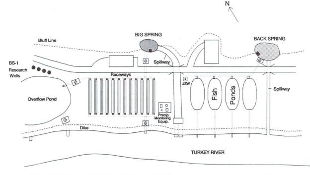
Figure 10. Diagram of Big Spring Hatchery. Dotted lines indicate structures that are underground.
