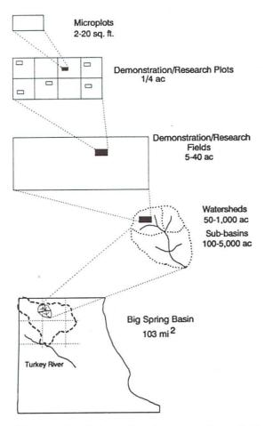
Figure 3. Schematic diagram of nested monitoring network design.
