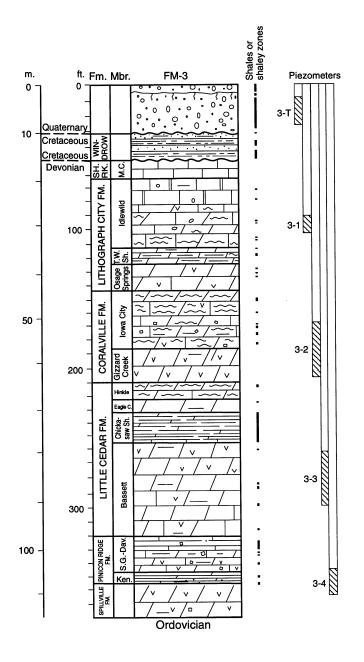
Figure 10. Geologic log, packer-test intervals, and piezometer completions, Site #3.
