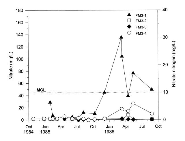
Figure 21. Nitrate concentrations at Site #3 bedrock piezometers.
