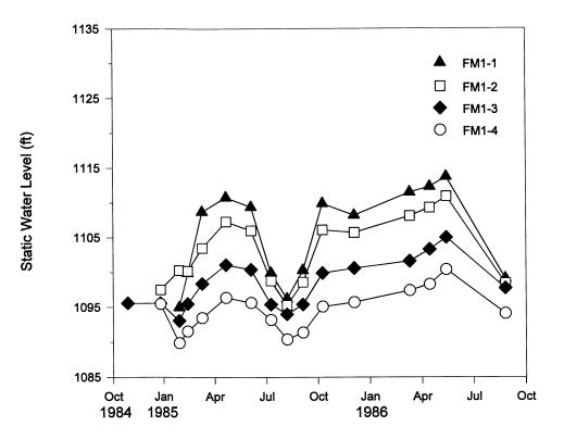
Figure 14. Potentiometric elevations at Site #1 bedrock piezometers.
