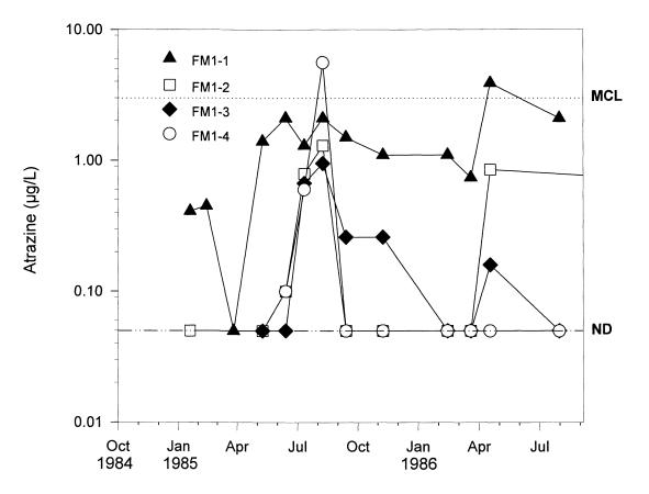
Figure 23. Atrazine concentrations at Site #1 bedrock piezometers.
