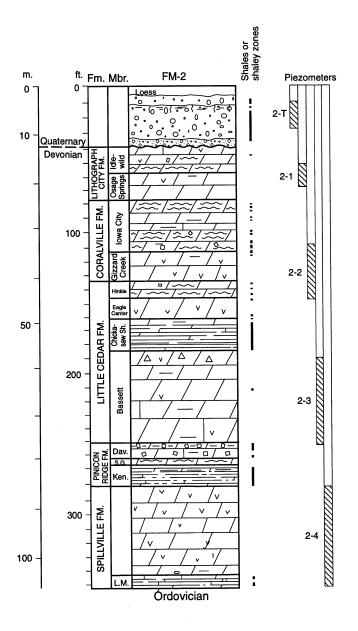
Figure 9. Geologic log, packer-test intervals, and piezometer completions, Site #2.
