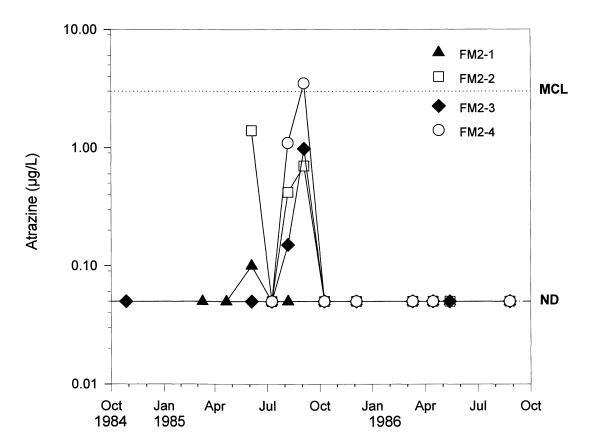
Figure 24. Atrazine concentrations at Site #2 bedrock piezometers.
