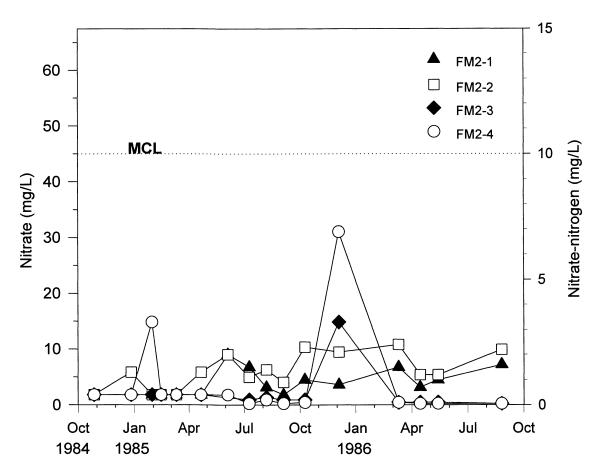
Figure 20. Nitrate concentrations at Site #2 bedrock piezometers.
