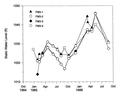
Figure 17. Potentiometric elevations at Site #3 bedrock piezometers.
