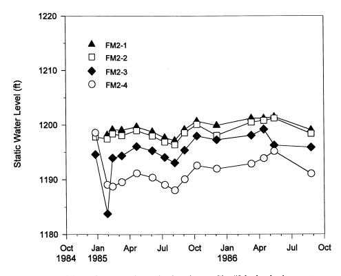
Figure 15. Potentiometric elevations at Site #2 bedrock piezometers.
