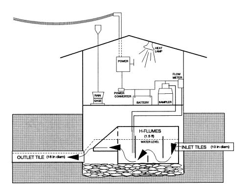
Figure 16. Diagram of the Bugenhagen sub-basin instrument shed.
