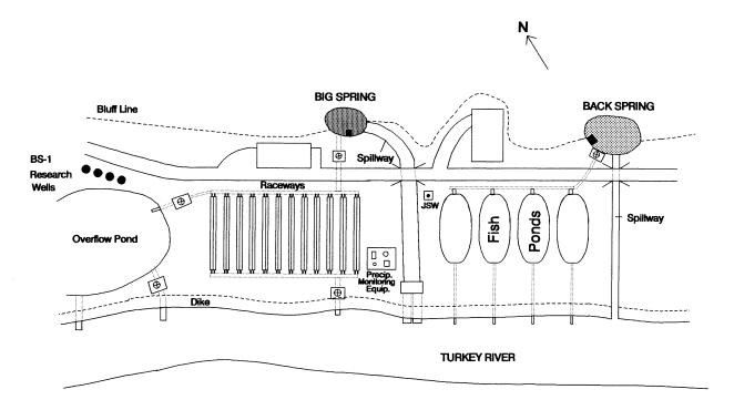
Figure 19. Diagram of Big Spring Hatchery and monitoring system. Dotted lines indicate structures that are underground.
